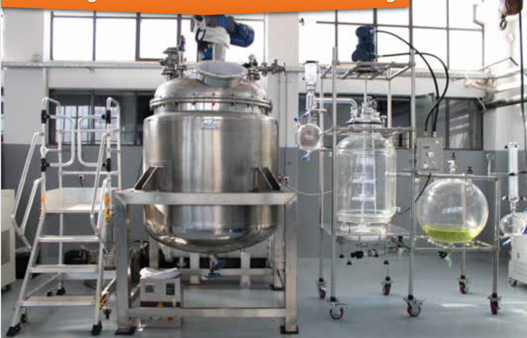
Leaching unit with conventional heating
